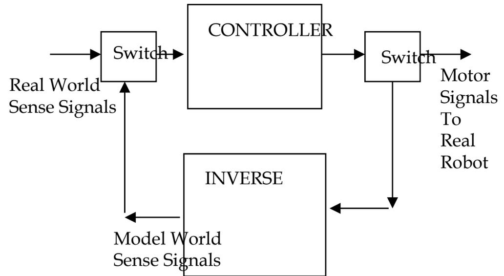
**Normal Mode** – controller produces motor signals, inverse detects mismatch or *novelty*.
